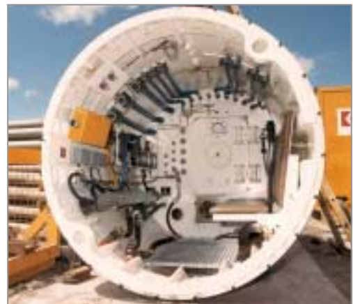
Picture 17: Air Lock
