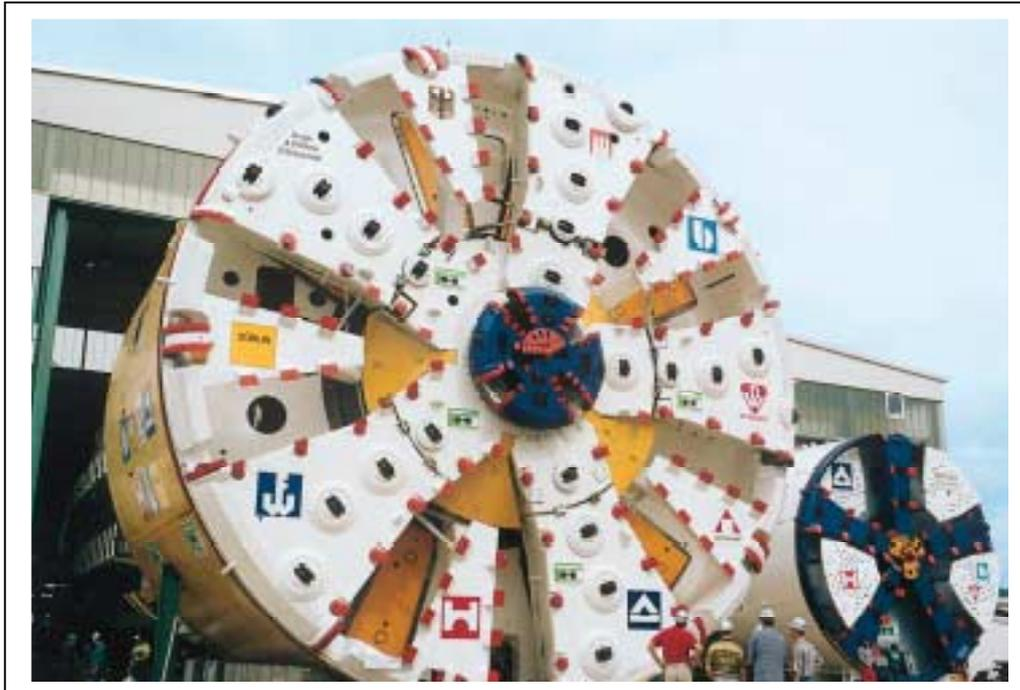
*Fig.2: Typical spoke type cutterhead of the Mixshield
