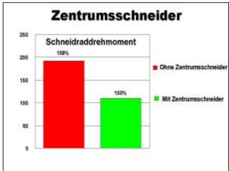
Fig. 7: Comparison cutterhead torque with/without
