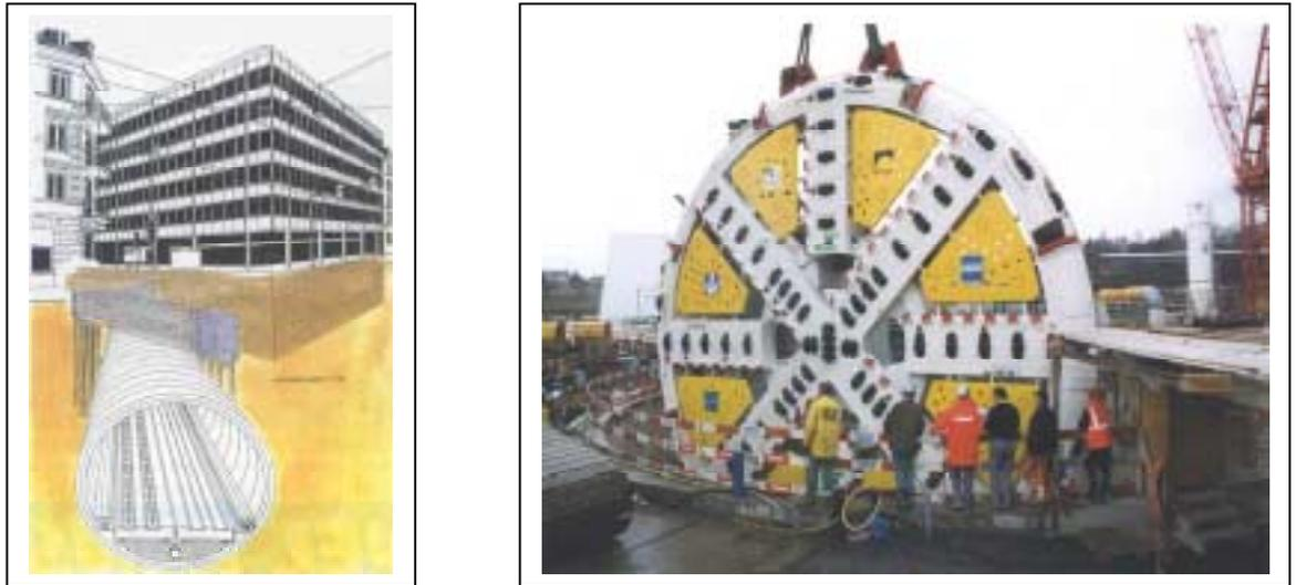
*Fig. 20: Mixschild for Zürich-Thalwil / Switzerland / ( $\varnothing 12,63$  m) at very low coverage (left picture)*
