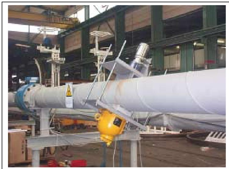
*Fig.10: Radiometric density and magnetic-inductive flow meters*
