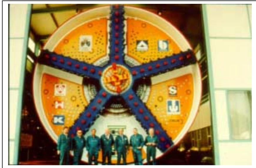
*Fig.16: Mixschild for Metro Essen /Germany / ( $\varnothing$  8,3 m) with active center cutter*
