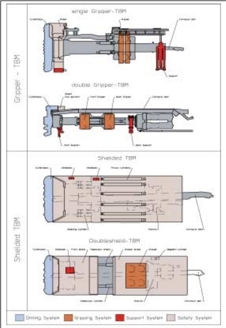
*Fig.3: Various types of hardrock TBM*
