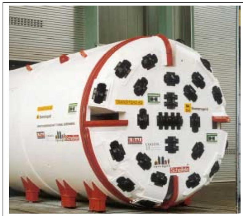
*Fig.6: Shielded TBM (Sörenberg Ø 4,56 m / Switzerland)*
