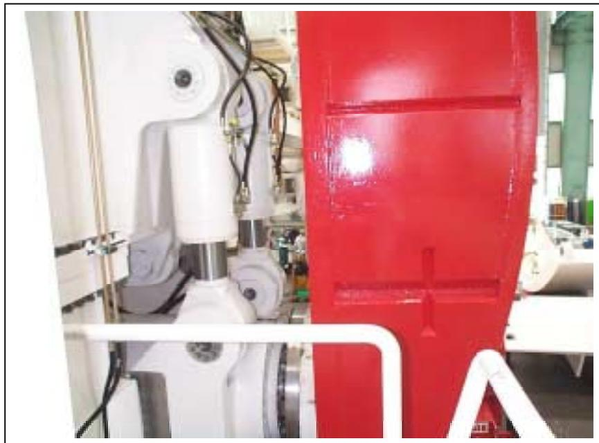
*Fig.5: Steering cylinder for a single gripper-TBM*
