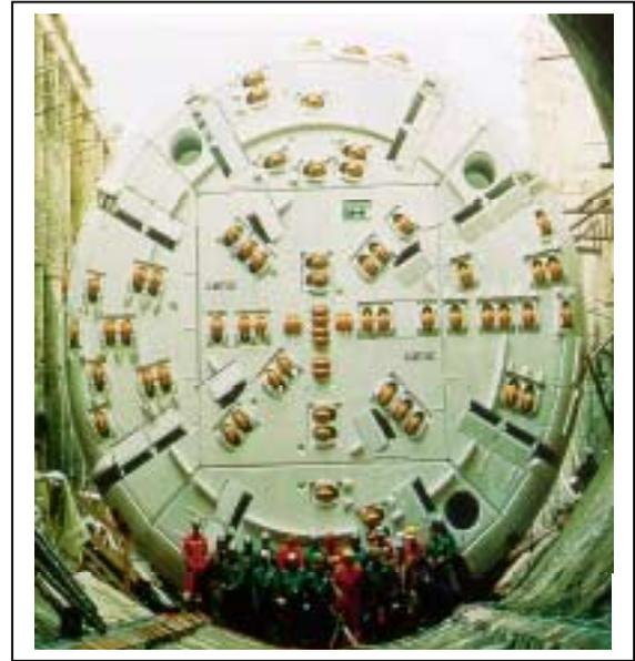
*Fig.14: Schielded TBM Murgenthal
