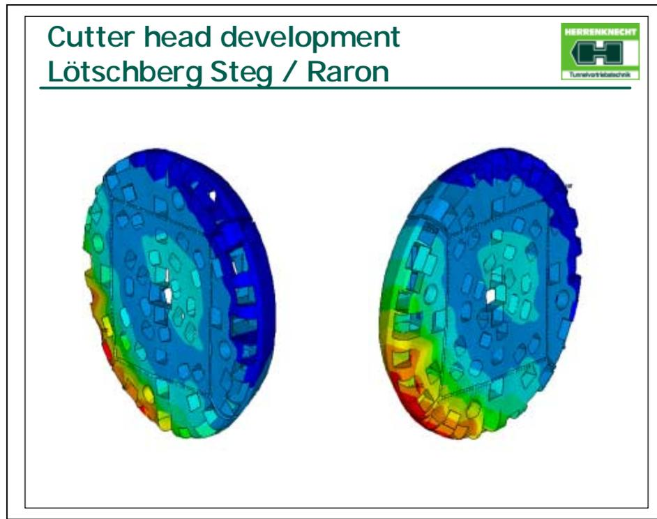
*Fig.9: F/E-modelling of the cutterhead*
