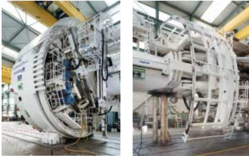
*Fig. 18: Mechanical equipment for excavation stabilisation, gripper-TBM S-167,
