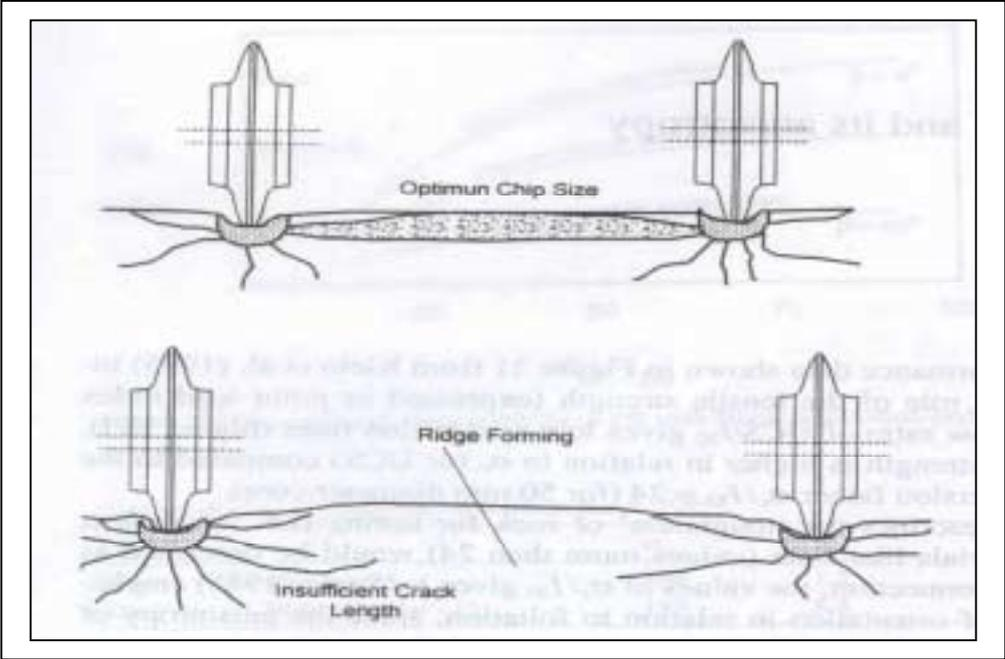
*Fig. 8: Chipping process between two disc cutters*
