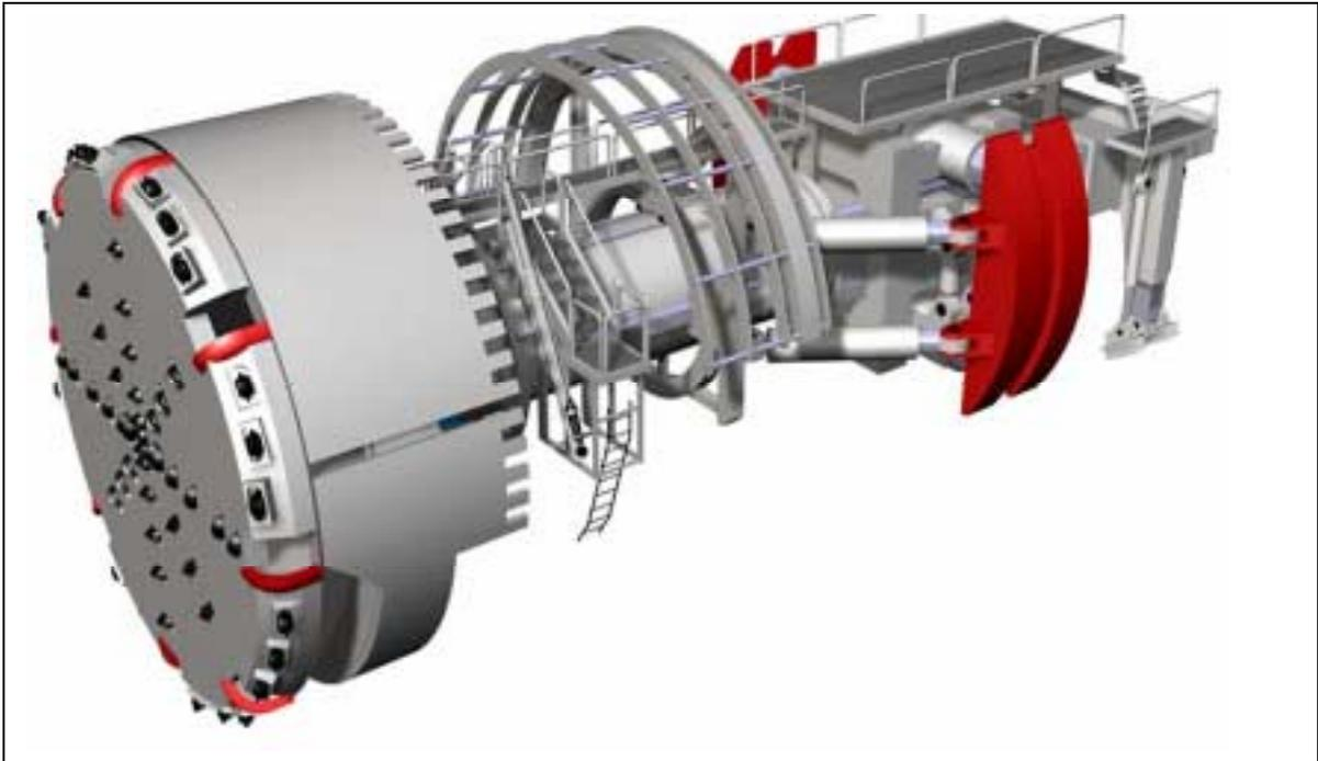
*Fig.4: Single gripper-TBM*
