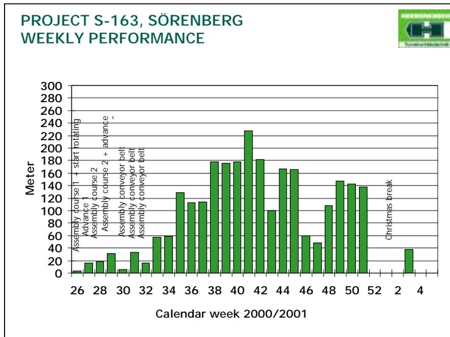
Fig. 12: Tunnelling performance shield TBM S-163, Sörenberg Tunnel, Ø 4.56 m
