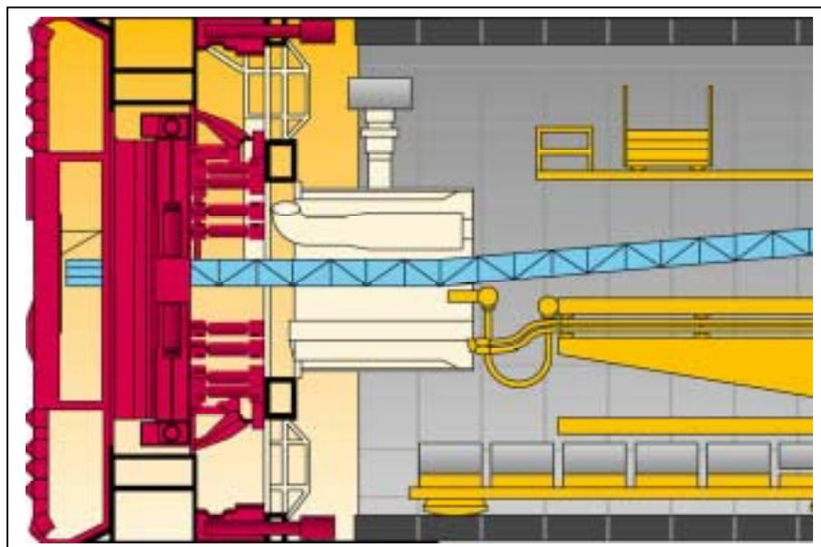
*Fig.2: Principle of a shielded hardrock TBM*
