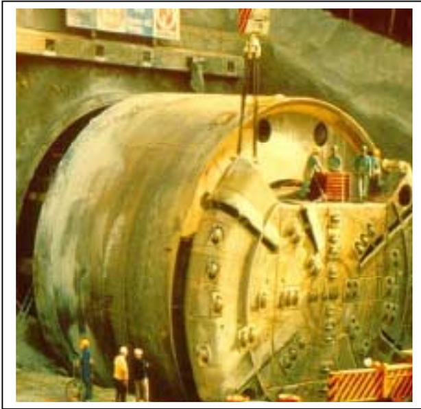
*Fig.13 Schieldeld TBM Bözberg
