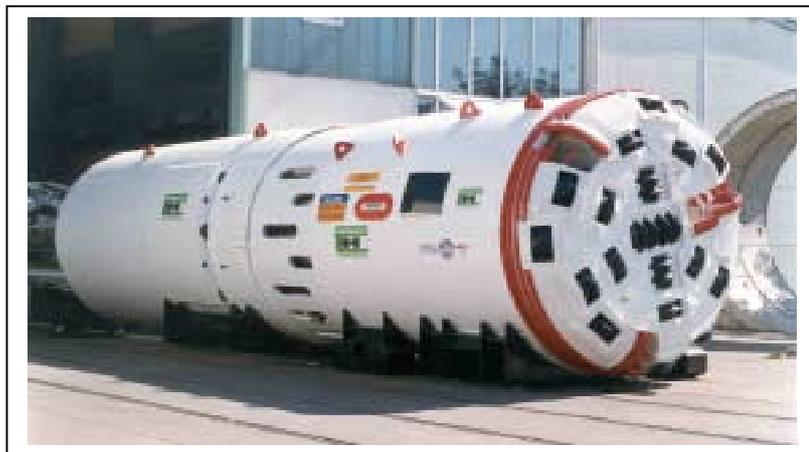
*Fig. 16: Double-shield TBM La Réunion  $\varnothing$  3.87 m*
