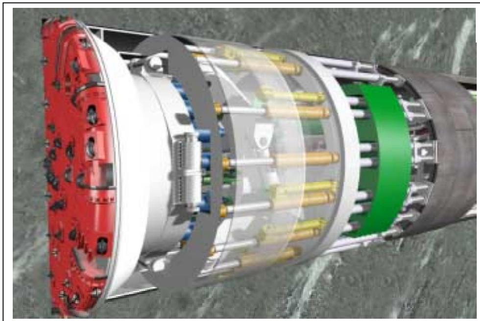
*Fig.7: Double-shield TBM*
