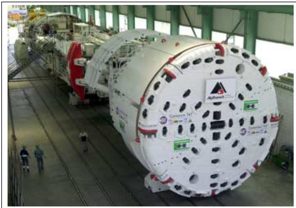
*Fig.1: Hardrock TBM for the longest Railway-Tunnel in the world
