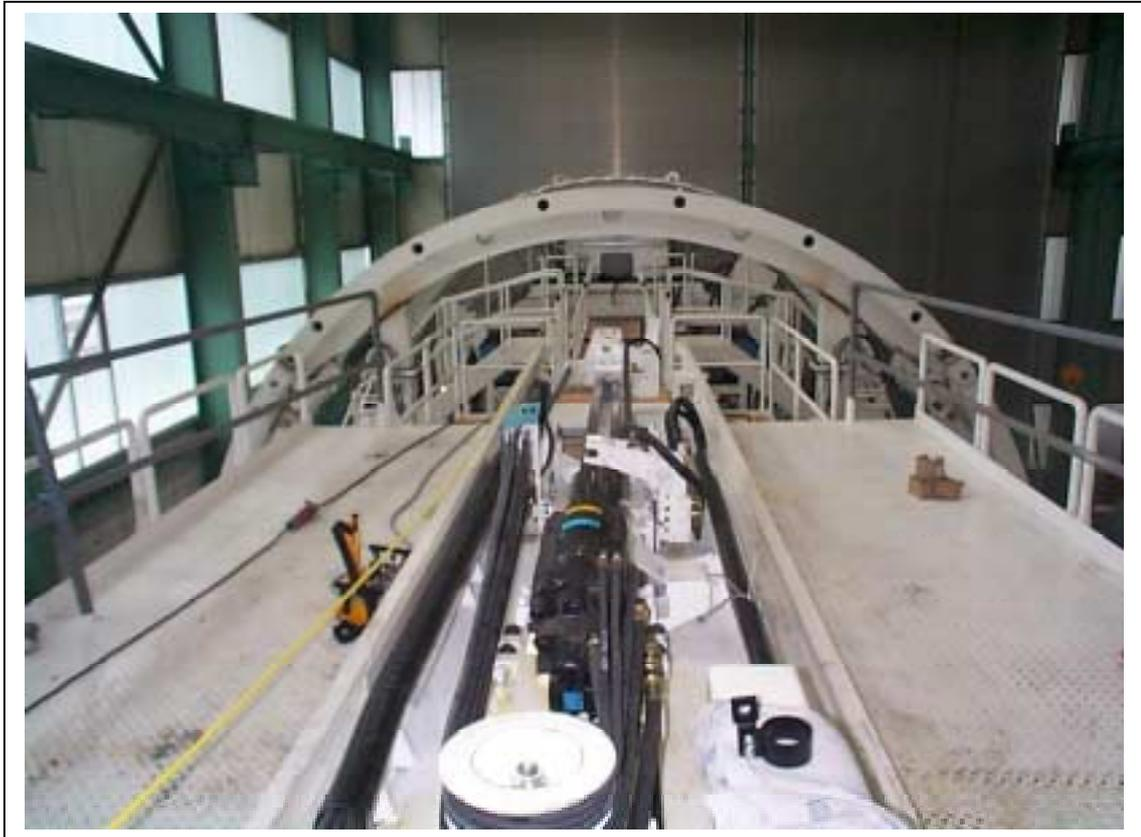
*Fig.11: Fixed installed probe/ injection drill device*
