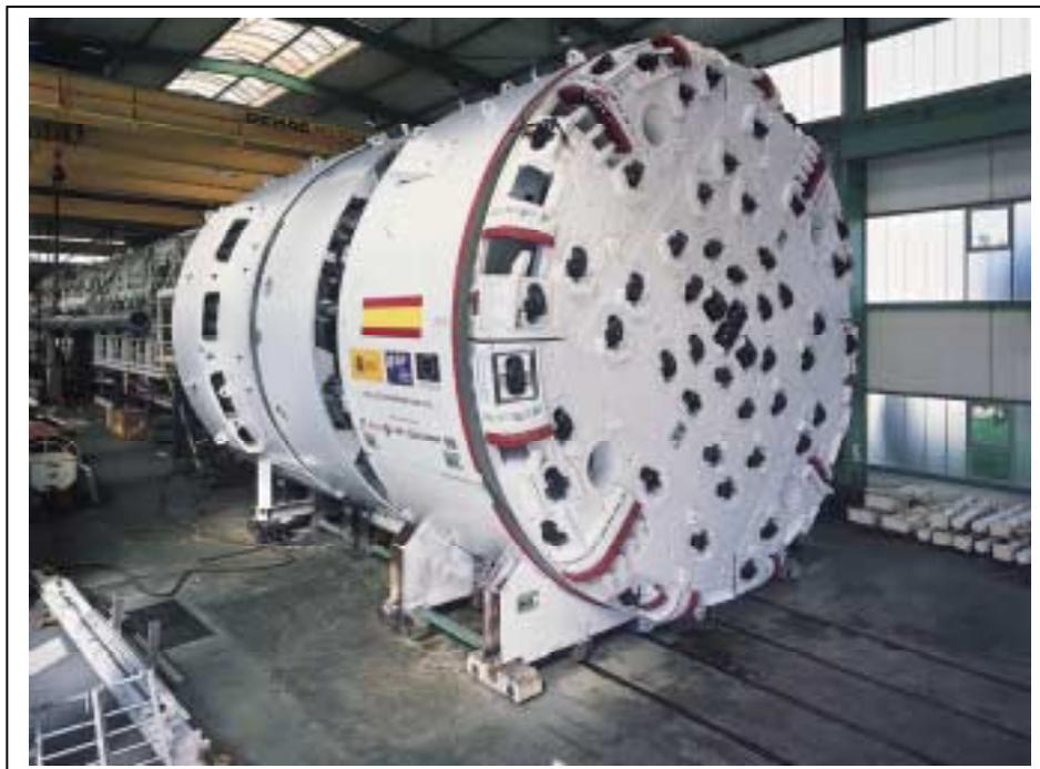
*Fig. 15: Double-shield TBM Guadarrama / Spain, Ø 9.51 m*
