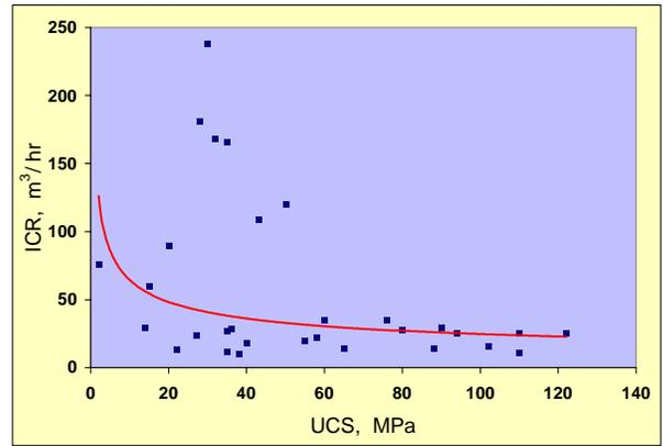
Figure-4: Plot of ICR Vs. UCS for Sedimentary Rocks and Transverse Roadheaders
