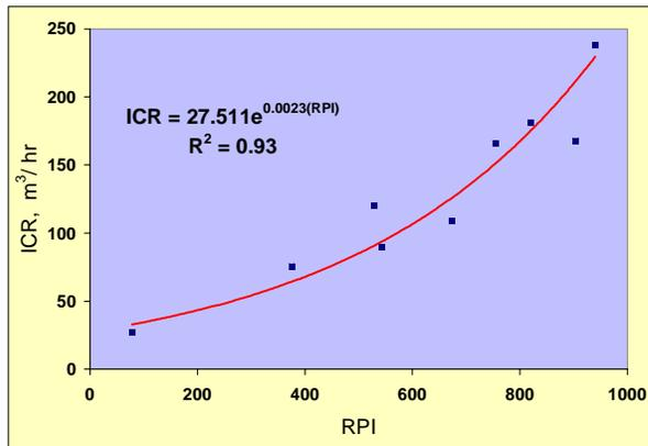
Figure-8: Plot of ICR Vs. RPI for Evaporitic Rocks and Transverse Roadheaders
