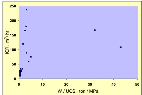
Figure-6: Plot of ICR Vs. W / UCS for Sedimentary Rocks and Transverse Roadheaders
