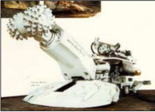
Figure-1: A Transverse Cutterhead Roadheader
