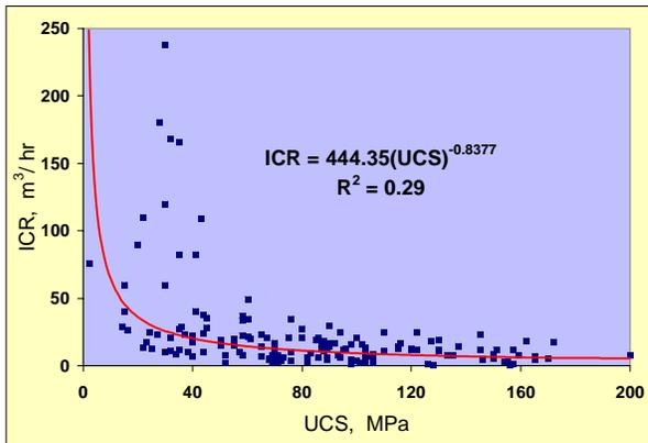
Figure-3: Plot of ICR Vs. UCS for All Geological Conditions and All Types of Roadheaders
