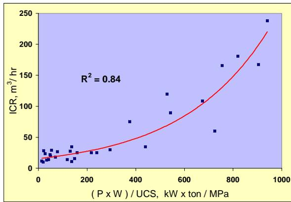
Figure-7: Plot of ICR Vs. (P x W / UCS) for Sedimentary Rocks and Transverse Roadheaders
