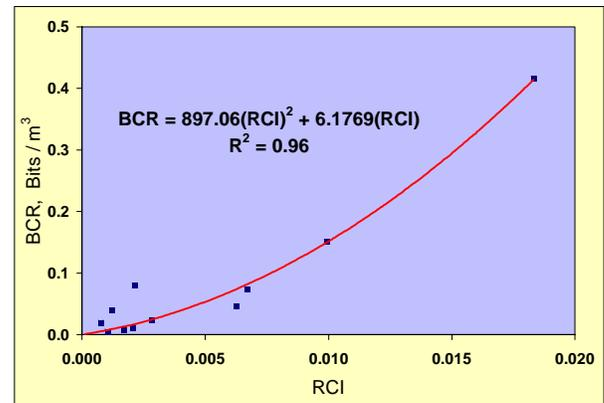
Figure-11: Plot of BCR Vs. RCI for Sedimentary Rocks and Transverse Roadheaders
