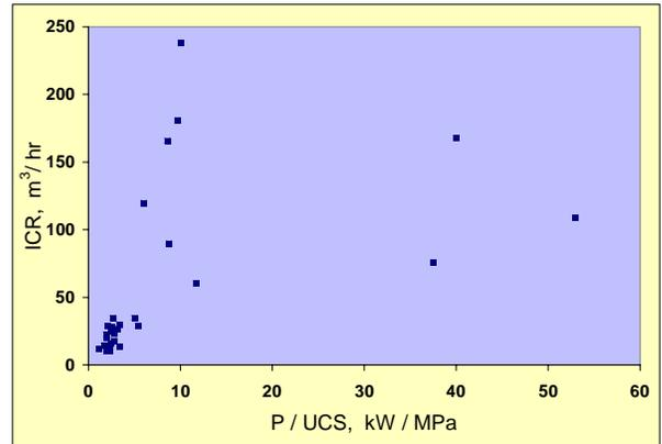
Figure-5: Plot of ICR Vs. P / UCS for Sedimentary Rocks and Transverse Roadheaders
