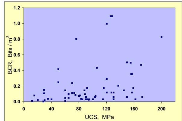
Figure-9: Plot of BCR Vs. UCS for All Geological Conditions and All Types of Roadheaders
