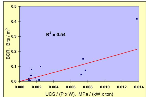
Figure-10: Plot of BCR Vs. UCS / (P x W) for Sedimentary Rocks and Transverse Roadheaders
