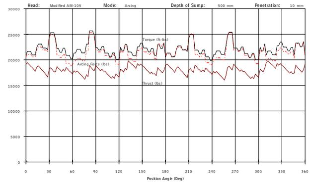
Figure 3. An example of vibration monitoring output, cutterhead thrust and torque variation.
