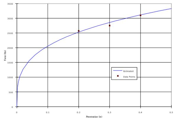
Figure 2. Estimated and measured normal forces.
