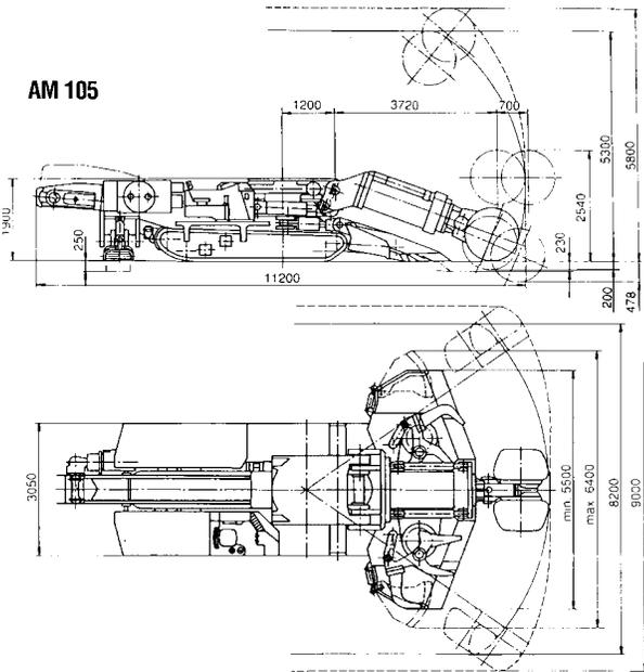
Figure 1. General Drawings of VA AM-105 roadheader
