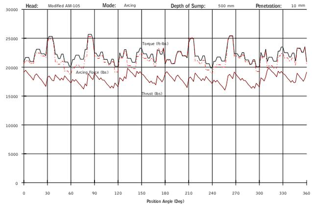
Figure 4. An example of vibration monitoring output, cutterhead thrust and torque variation.
