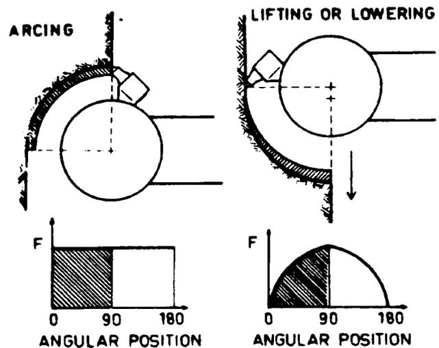
Figure 2. Shape of cutting area of the bits in various cutting modes (After Hekimoglu 1991).
