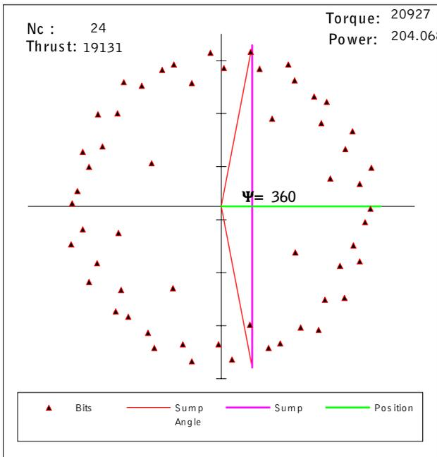
Figure 1. Plan view of the cutterhead bit layout pattern (with 115° angular spacing).
