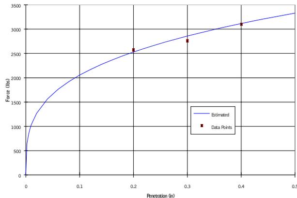
Figure 3. Estimated and measured normal forces.
