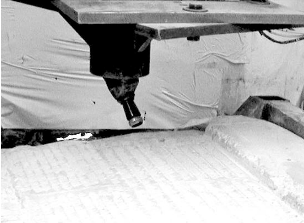
Figure 12: 38 mm Frustum Cutting Lyons Sandstone.
