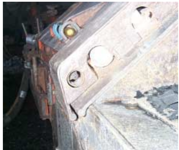
Figure 11: Headlamp spray assembly.
