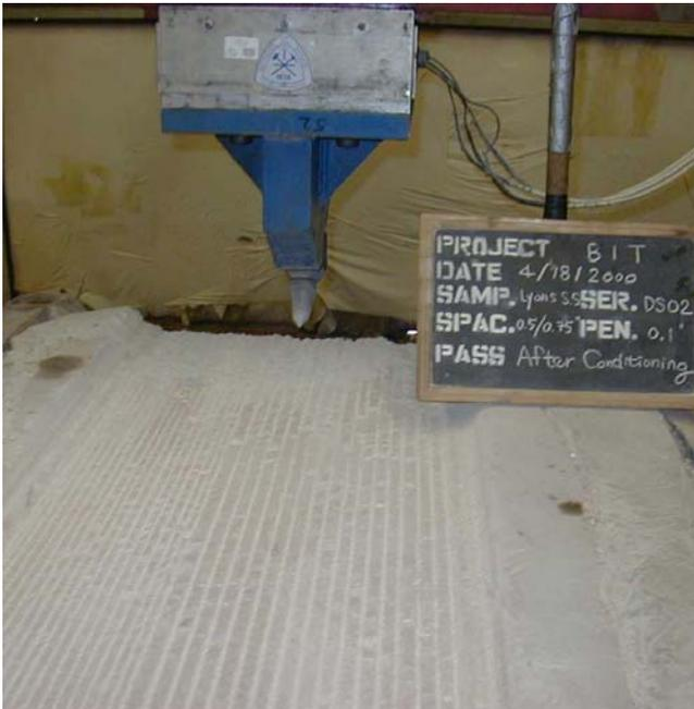
Figure 10: Sample during for linear cutting tests.
